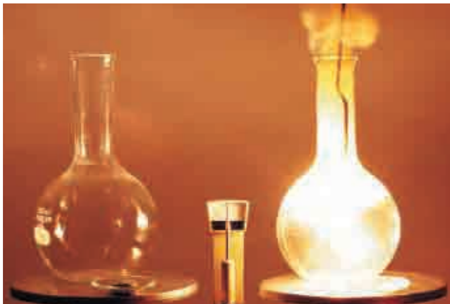
Figure 12.14 In this photograph, oxygen gas reacts with calcium to produce calcium oxide.
