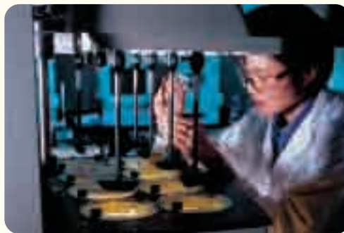
An analyst tests whether tablets will sufficiently dissolve within a given time limit.
