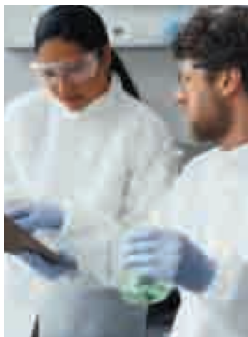
Figure 8.24 When diluting acid, always add the acid to the water—never the reverse. Rubber gloves, a lab coat, and safety goggles or a face shield protect against acid splashes.
