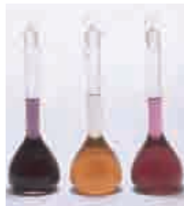
Figure 8.19 These volumetric flasks, from left to right, contain solutions of chromium(III) salts, iron(III) salts, and cobalt(II) salts.
