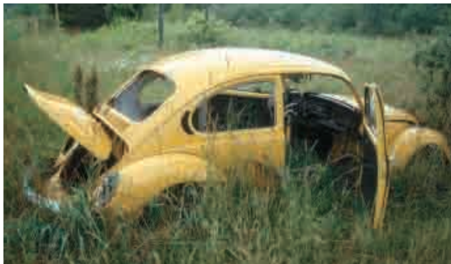
Figure 4.6 The iron in this car undergoes a synthesis reaction with the oxygen in the air. Iron(III) oxide, also known as rust, is formed.
