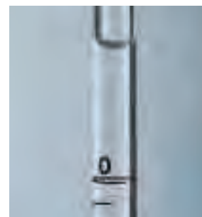
Figure 10.16 Draw a bit more liquid than you need into the pipette. It is easier to reduce this volume than it is to add more solution to the pipettes.
