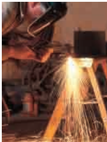
Figure 14.6 The combustion of acetylene (ethyne) in an oxyacetylene torch produces the highest temperature (about 3300°C) of any known mixture of combustible gases. Metal workers can use the heat from this combustion to cut through most metal alloys.
