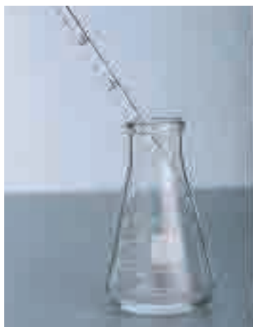
Figure 10.18 You can prevent a “stubborn” drop from clinging to the pipette tip by touching the tip to the inside of the glass surface.
