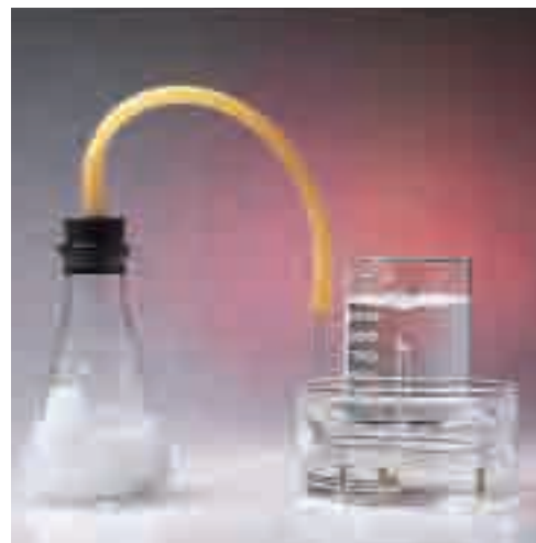
Figure 12.16 This is an efficient and convenient method for collecting hydrogen gas. Unfortunately molecules of water vapour mix with the gas sample.
