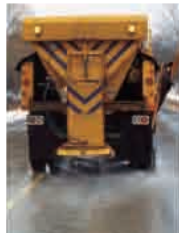
Figure 3.2 Sodium chloride is used to melt ice because salt water has a lower melting point than pure water.
