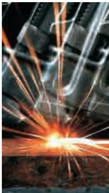
The thermite reaction generates enough heat to melt the elemental iron that is produced.
