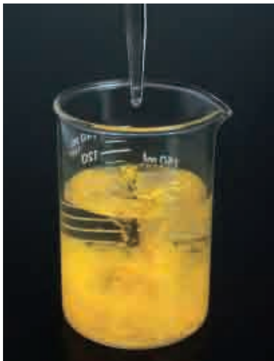
Figure 9.4 Lead(II) nitrate and potassium iodide are clear, colourless aqueous solutions. Mixing them causes a double displacement reaction. An insoluble yellow precipitate (lead(II) iodide) and a soluble salt (potassium nitrate) are produced.
