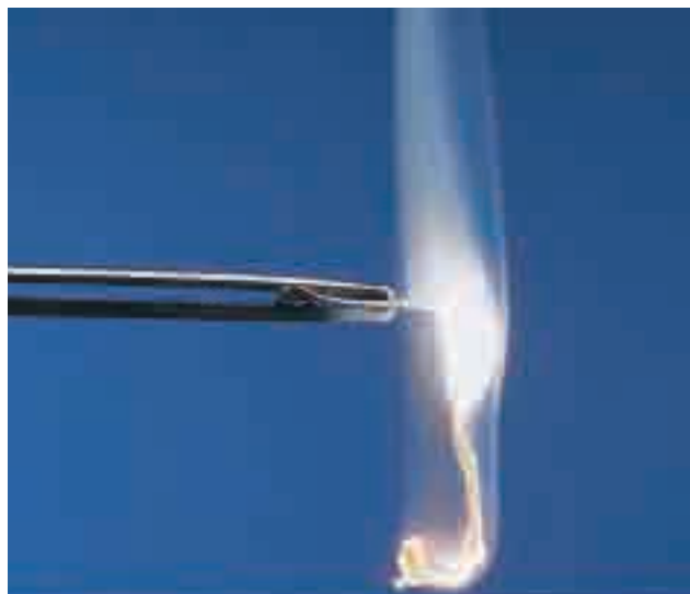
Figure 4.11 Magnesium metal burns in oxygen. The smoke and ash that are produced in this combustion reaction are magnesium oxide.
