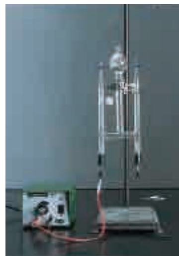
Figure 1.10 An electrical current is used to decompose water. This process is known as electrolysis.
