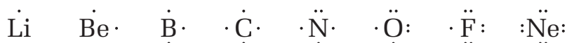
Figure 2.11 Examine these Lewis structures for the Period 2 elements. Place a dot on each side of the element—one dot for each valence electron. Then start pairing dots when you reach five or more valence electrons.
