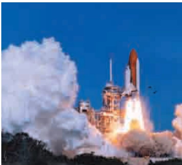
Figure 11.30 The large centre tank that is attached to the shuttle orbiter has two compartments, one containing liquid hydrogen and the other containing liquid oxygen. The energy released by the reaction between these two substances provides the thrust needed to propel the orbiter into space.
