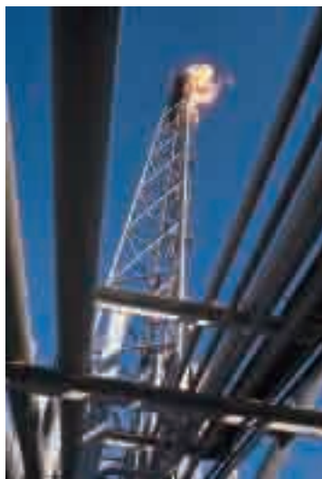
Figure 14.2 Sour gas, \text{H}_2\text{S}_{(g)} , is sometimes “flared off” (burned) from an oil well. This combustion produces sulfur dioxide gas, which reacts with the water in the atmosphere to produce acid rain. Oil companies are now making an effort to reduce this type of pollution.
