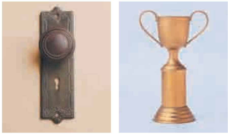
Figure 8.16 Brass can be made using any percent from 50% to 85% copper, and from 15% to 50% zinc. As a result, two objects made of brass can look very different.
