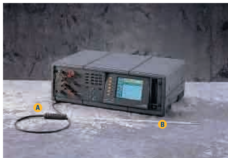
Figure 1.6 These two thermometers measure the same temperature. Thermometer A is calibrated into divisions of 0.1°C. Thermometer B is calibrated into divisions of 1°C. Which thermometer lets you make more precise measurements? Which digits in each thermometer reading are you certain about? Which digits are you uncertain about?
