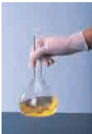
Figure 8.21 Add distilled water until the flask is about half full. Swirl the mixture around in order to dissolve the solute completely. Rinse the beaker that contained the solute with solvent. Add the rinsing to the flask.
