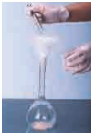
Figure 8.20 Transfer a known mass of solid solute into the volumetric flask. Alternatively, dissolve the solid in a small volume of solvent. Then add the liquid to the flask.
