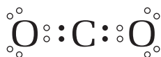
Figure 3.18 This Lewis structure shows the double bond in a molecule of carbon dioxide, \text{CO}_2 .
