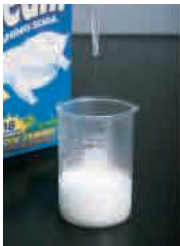
Figure 4.17 The reaction of hydrochloric acid and sodium carbonate, Na 2 CO 3 (washing soda), is a double displacement reaction. This reaction initially forms sodium chloride and carbonic acid, H 2 CO 3 . The carbonic acid spontaneously decomposes to water and carbon dioxide gas.
