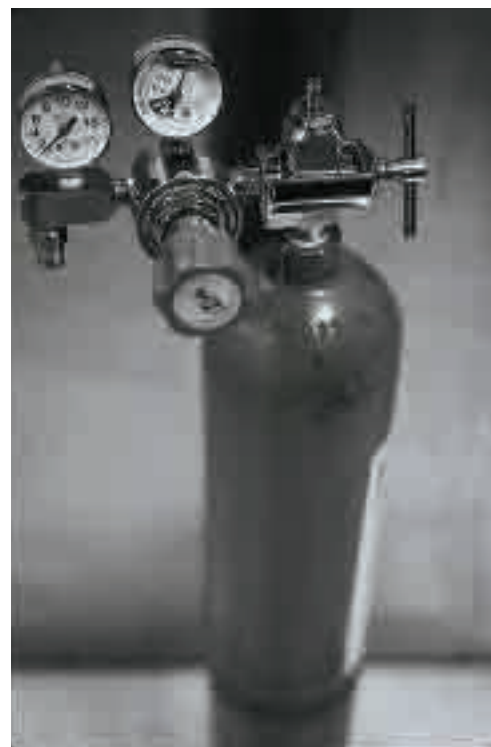
Figure 11.22 Pressure relief valves prevent a compressed gas cylinder from exploding if the temperature, and thus the pressure increases.
