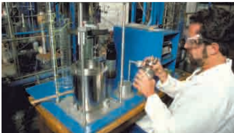
Figure 14.19 Bomb calorimeters give more accurate measurements than polystyrene calorimeters.
