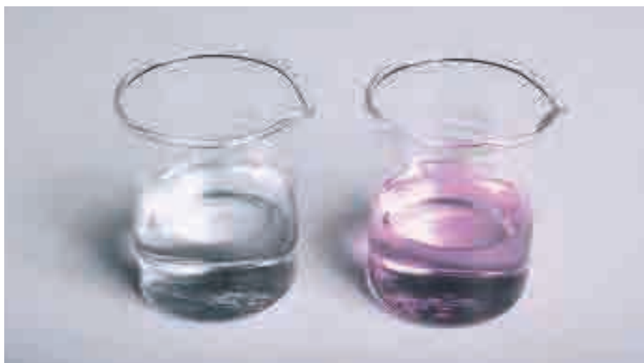
Figure 10.14 A good indicator, such as the phenolphthalein shown here, must give a vivid colour change.
