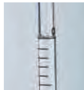
Figure 10.17 The bottom of the meniscus must align exactly with the etched mark.
