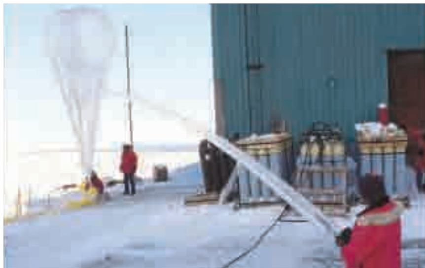
Figure 11.11 Weather balloons are partially inflated with helium. They carry specialised instruments to measure varying atmospheric conditions such as pressure, temperature, and humidity.
