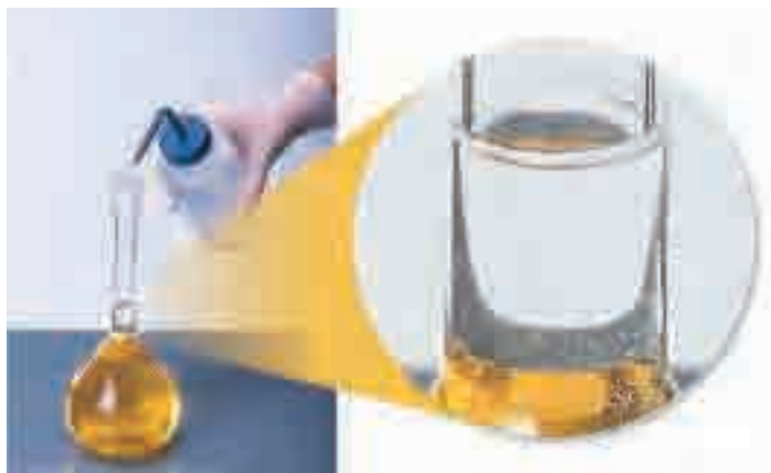
Figure 8.22 Add the rest of the water slowly. When the flask is almost full, add the water drop by drop until the bottom of the meniscus rests at the etched line.
